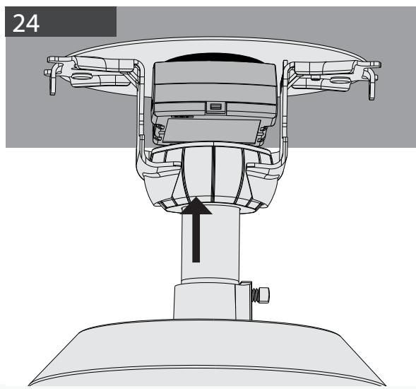
Place receiver in ceiling bracket. Excess wire may be placed into the outlet box for non-concrete ceilings or inside the hanger bracket for concrete ceilings.
