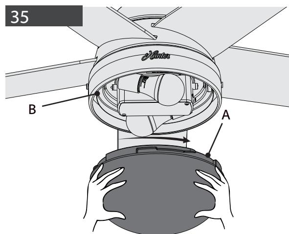
Lift the globe and align the notches (A) in the globe with the tabs (B) in the light kit. Attach the glass bowl to the light kit by twisting it clockwise until it snaps into place.
