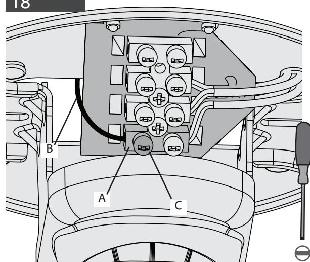
This is the procedure for steps 19-23. Thread the end of each wire into the terminal block (A) on the hanger bracket, then secure each supply main (B) by tightening the small setscrews (C).
