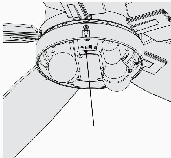
**English** **Changing the bulbs** - rotate the globe counter clockwise and lower once released from the tabs. Replace bulbs with bulbs of the same type and wattage. Reinstall the globe.
