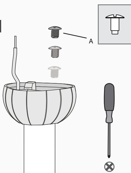
Insert the downrod ball screw (A) into the hole in the top of the downrod ball.
