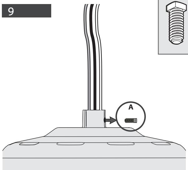
Remove the pre-installed setscrew (A).
