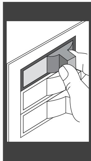
**English** To access the battery compartment, remove the battery door from the transmitter assembly. The battery should be installed with the positive (+) side up. Replace with a CR2032 battery when necessary.
