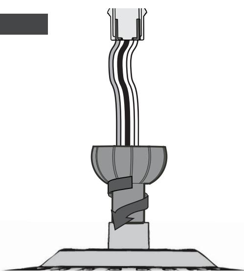
Hand tighten the downrod (at least 4-5 full turns) until it stops.
