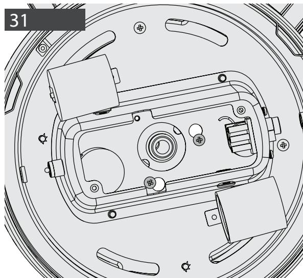
Feed the 9-pin plug connector coming from the bottom of the motor housing through the center hole in the light kit assembly. Connect it to the plug connector found in the switch housing area of the light kit assembly. Make sure to line up the colored markings on the connectors.
