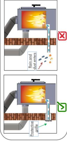
External air intake vents air into the combustion chamber. This is mandatory to use in buildings that are very airtight (buildings with non-closable vents). If external air intake cannot be used then there must be an space of at least 10 cm between the stove and the rear wall so the appliance functions correctly.
