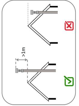
2°.- Chimney cap above the highest part of the roof ridge but with a taller building close
