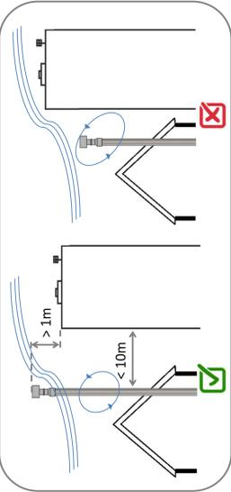
3°.- Chimney cap installed at the end of the smoke outlet
