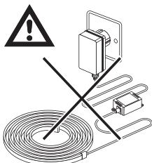
Do not connect the rope light to the supply while it is wound onto a reel.
