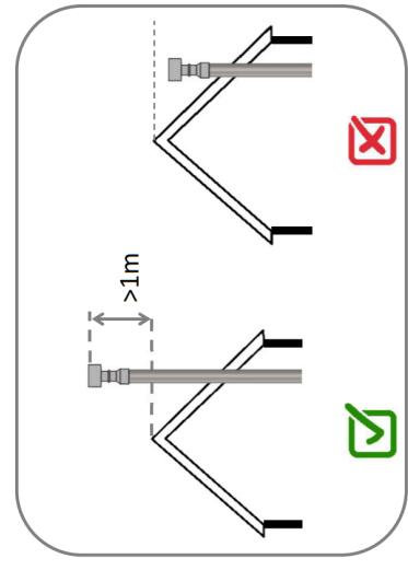
**2º.- Chimney cap above the highest part of the roof ridge but with a taller building close**
