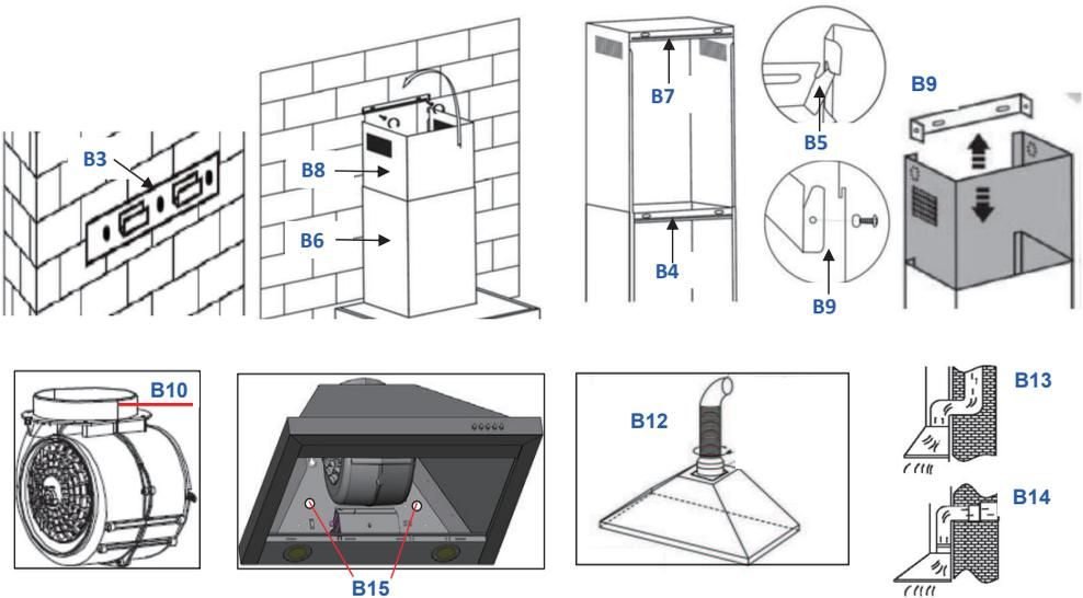
15. Hang the cooker hood on the suspension plate **B3** again and secure it well by fixing the screws through the 2 holes **B15** on the wall, so that the hood can not accidentally be removed from the wall.
