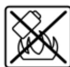
**Protect the battery against heat, e. g. against continuous intense sunlight, fire, dirt, water and moisture.** There is a risk of explosion and short-circuiting.
