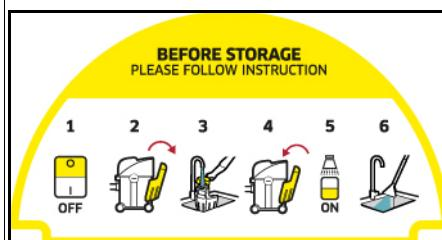
There is a label on the storage space of the device that describes how to clean the device before storing it:
