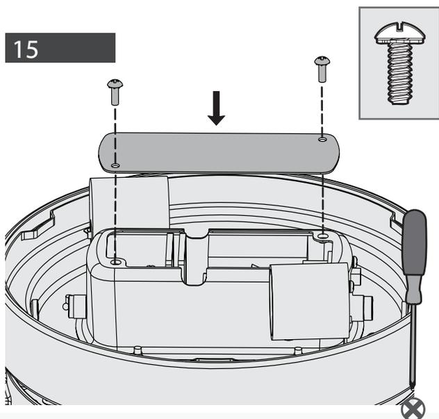
Carefully push all switch housing components into the switch housing, then install the switch housing plate using two light kit assembly screws, found in the
