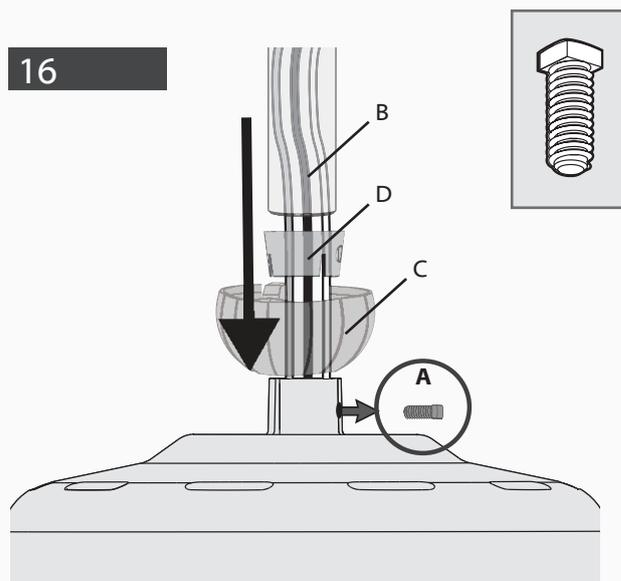
Remove the pre-installed setscrew (A) so that the downrod (B) can be inserted. Save the setscrew (A). Guide the downrod (B), sleeve (D), and downrod (B) down the wires coming from the fan.
