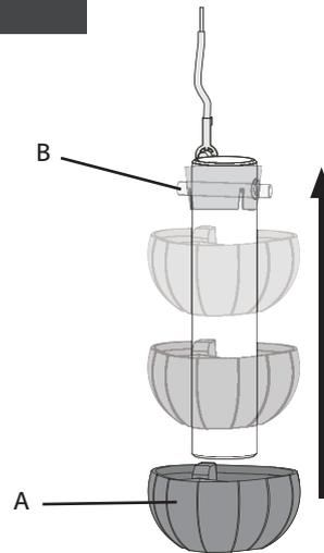
Slide the downrod ball (A) up the length of the downrod pipe. Align the downrod pin (B) with the notches in the downrod ball (A).
