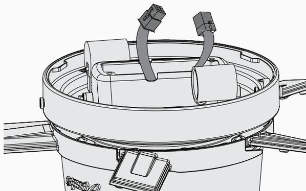
Feed the 9-pin plug connector coming from the bottom of the motor housing through the center hole in the light kit assembly. Connect it to the plug connector found in the switch housing area of the light kit assembly. Make sure to line up the colored markings on the connectors.
