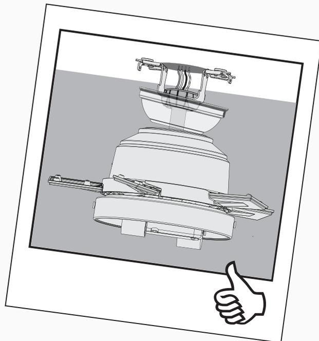
**English** **DO NOT PICK THE FAN UP BY THE CANOPY OR WIRES.** Place the downrod ball into the slot in the ceiling bracket.
