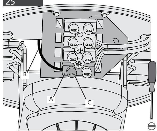
This is the procedure for steps 19-23. Thread the end of each wire into the terminal block (A) on the hanger bracket, then secure each supply main (B) by tightening the small setscrews (C).
