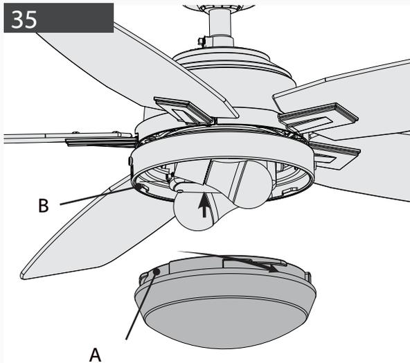
Lift the globe and align the notches (A) in the globe with the tabs (B) in the light kit. Attach the glass bowl to the light kit by twisting it clockwise until it snaps into place.
