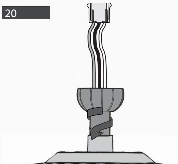
Hand tighten the downrod (at least 4-5 full turns) until it stops.
