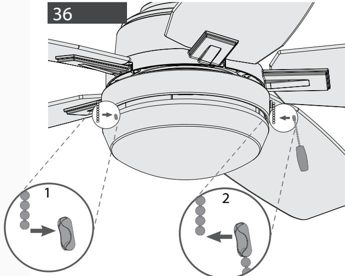
1. Remove and discard the plastic connectors from the ends of the short pull chains coming from the sides of the light kit assembly.
