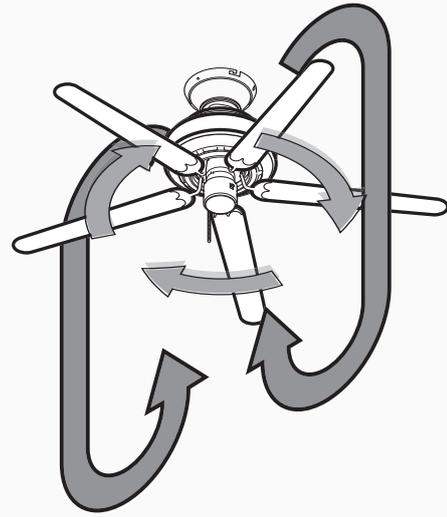
**English** In warm weather, ceiling fans work best by blowing air downward (counterclockwise) providing the room with a cool breeze.
