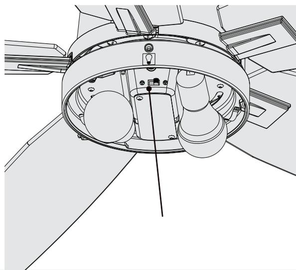
**Changing the bulbs** - rotate the globe counter clockwise and lower once released from the tabs. Replace bulbs with bulbs of the same type and wattage. Reinstall the globe.
