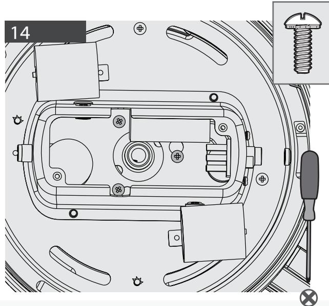
Insert a third light kit assembly screw, found in the hardware bag, into place and tighten all three screws securely.
