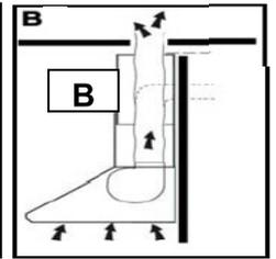
**B Installation for exhaust air mode**
