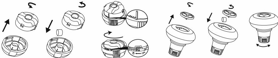
**IMPORTANT:** Don't use granulate tablets or throw the tablet directly in the water. The chemicals can deposit on the bottom, damage the material and discolor the PVC.
