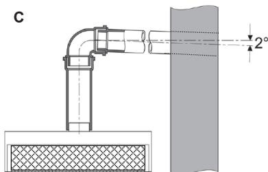
Otherwise condensation water could run into the extractor hood motor.
