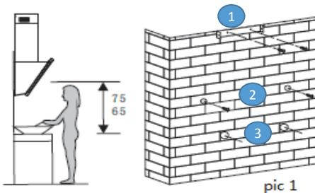
1. Drill 6pcs  $\varnothing 8$  mm holes in the wall at a suitable place to fix inside chimney hood body and safety screws once the installation height is fixed, and keep it in line. The installation position of the inside chimney bracket is the highest position of the inside chimney, see pic 1.
