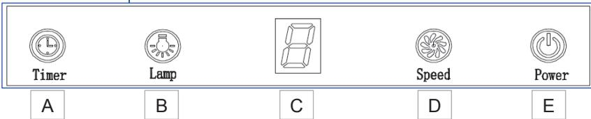
1. Press the "Power" button **E** , the button control the "ON/OFF" of the hood.
