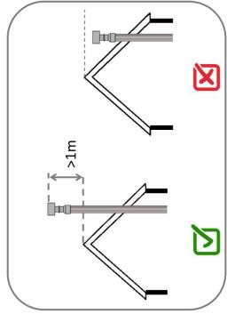
2°.- Chimney cap above the highest part of the roof ridge but with a taller building close
