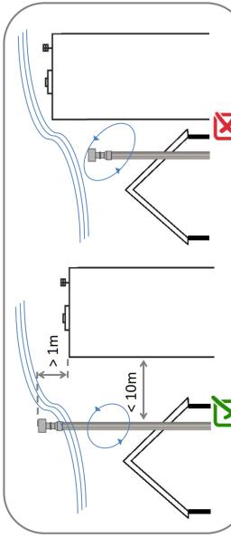
3°.- Chimney cap installed at the end of the smoke outlet
