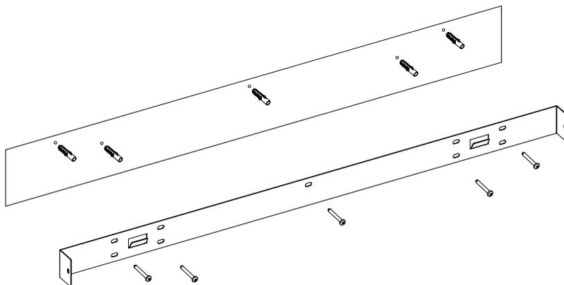
**2.1D** Use four ST4 x 8 screws to fix the L brackets to the base plate of the fireplace. Hang the fireplace on the brackets and mark the two holes for the L brackets on the wall. Then take down the fireplace. Drill two holes with an 8 mm drill bit at the marked locations. Then use the plastic dowels. Fix the fireplace to the bracket with two ST4 x 8 screws. Use two ST5 x 40 screws to fix the L brackets to the wall.
