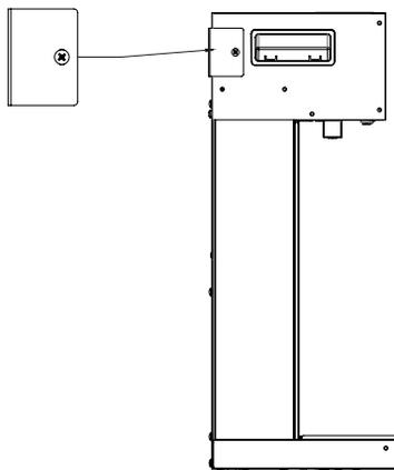
**2.1B** Decide on a stable wall and mount the mounting strip in the position where you want to hang the electric fireplace. After aligning the bracket, mark five drill holes on the wall. Drill the five holes for the appropriate dowel size that you want to use for mounting purposes.
